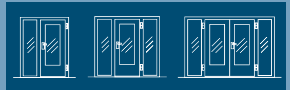
Floor to ceiling glazed doors without over-lights shown as single or double door arrangements
