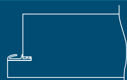
Non-standard rebate with cover sealing
